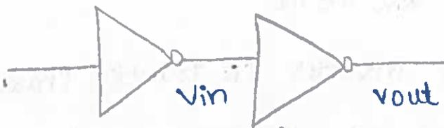
Fig: nmos inverter driven directly by another inverter.
